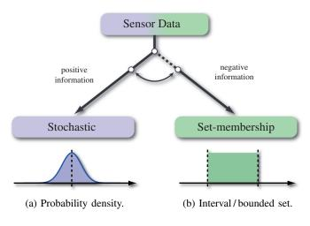
Fig. 1: Switching sensor noise model.
