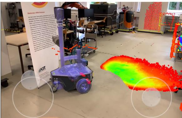
**Fig. 6:** Example teleoperation of a Gammabot (blue) from KIT-IPR, a ROBDEKON partner, using an iPad in AR. The captured point cloud is overlaid in real time.
