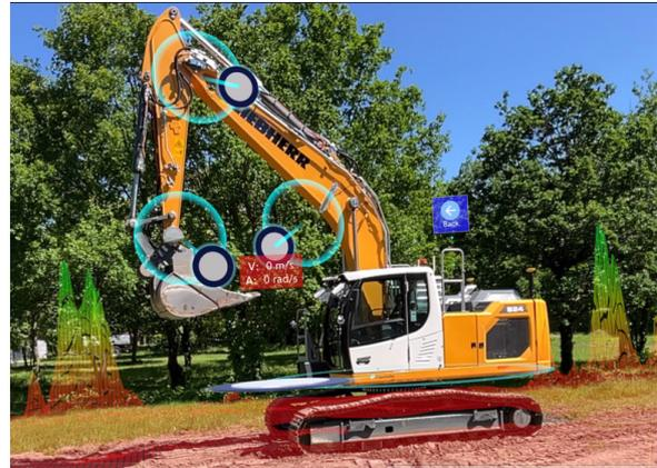
**Fig. 7:** Live teleoperation of an excavator from Fraunhofer IOSB, a ROBDEKON partner, with an iPad. The excavator’s joints can be controlled individually by spinning the markers in blue.
