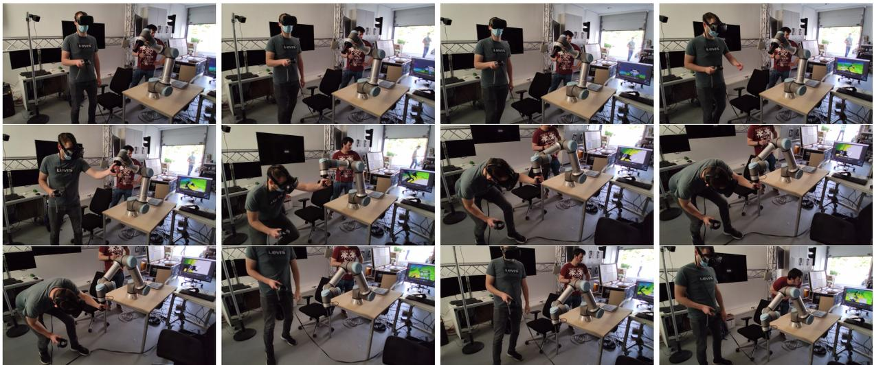
**Fig. 13:** Interaction of the user with the haptic robot during the trajectory selection process. The frames are approximately synchronized with those shown in Fig. 12.
