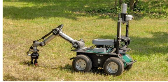
**Fig. 11:** The modified Husky robot from FZI used during the test deployment is shown grabbing a golf ball representing a contaminant. The box on top is considered as the safe containment.
