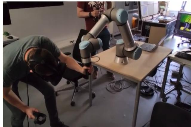
**Fig. 2:** Physical setup of the control station. A teleoperator with a VR headset operates a haptic robot (UR16e) that is programmed with haptic rendering to behave like a remote UR5.
