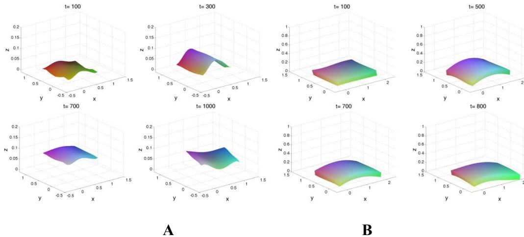
Fig. 3. Reconstruction over time of the thin membrane (Fig. 2A) with 36 measurement points and of the thick membrane (Fig. 2B) with 48 measurement points.
