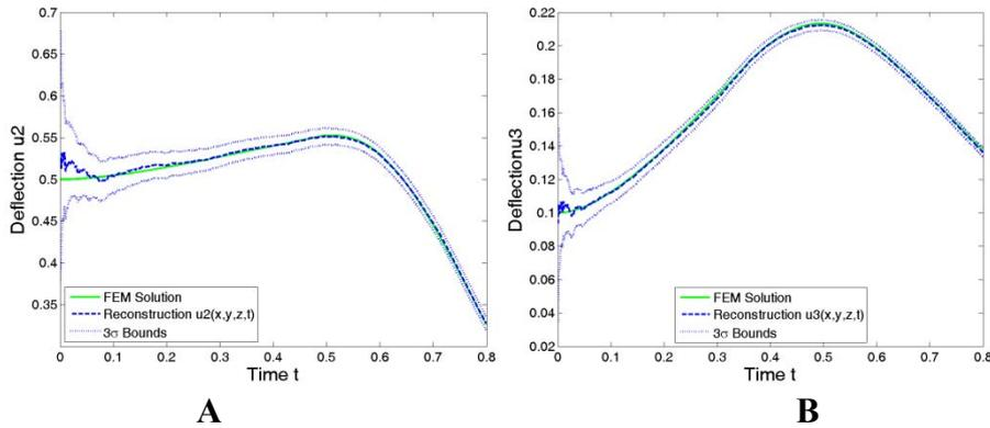
Fig. 2. Reconstruction at a non-measurement point for the thick membrane in direction y (Fig. 2.A), and in direction z (Fig. 2.B)
