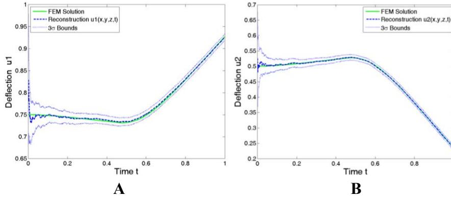
Fig. 1. Reconstruction at a non-measurement point for the thick membrane in direction x (Fig. 1A), and in direction y (Fig. 1.B).
