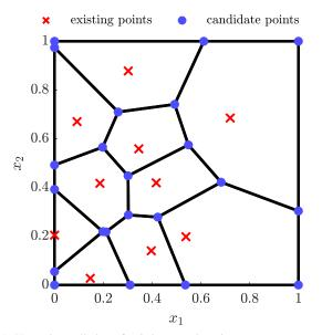
Fig. 1: Voronoi tessellation of existing sample points  $\underline{x}_i$ ,  $i = 1, \ldots, m$  (red crosses) and candidate points  $\underline{x}_j^{\text{cand}}$ ,  $j = 1, \ldots, N$  (blue dots) in a 2D design space. The candidate points are located at the corners of the Voronoi cells.
