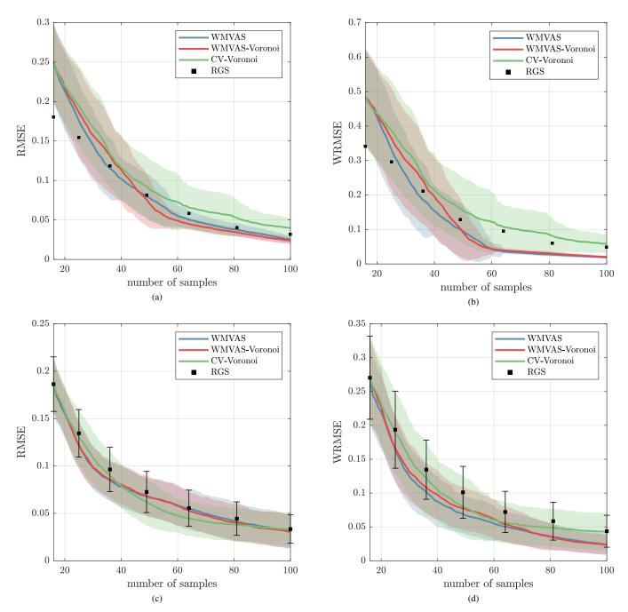
Fig. 4: Mean (solid lines, squares) and standard deviation (shaded areas, error bars) of the error measures (RMSE, WRMSE) vs. the number of samples. In 4a and 4b 100 runs were performed on the distribution in Fig. 2, where the algorithms were initialized with 16 random samples in each run. For 4c and 4d the algorithms were applied to 100 different distributions (one run per distribution). The same 16 initial grid points were used for each run.
