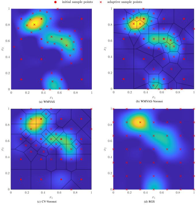
Fig. 3: Visualization of the meta model of the examined algorithms, evaluated on the two-dimensional design space. The space-filling initial points (red dots) and the adaptive points (red crosses) are shown on top. For the Voronoi-based approaches in Fig. 3b and 3c, the black lines represent the edges of the voronoi cells. The top row shows the proposed methods.
