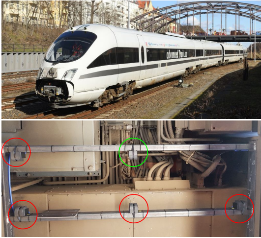
Figure 4. (top) Advanced TrainLab of the Deutsche Bahn. The advanced TrainLab is a diesel-electric train with a distributed traction concept. (bottom) Magnetometer array with five sensors. The different sensors are highlighted with circles. In this paper the sensor in the top middle (green circle) is used.
