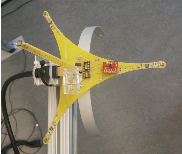
Fig. 4. A microphone array in tetrahedral shape mounted on a rail for testing. In the middle, a 3-axis-gyroscope is supplied to be fused with the acoustic tracking system. Microphones as well as the gyroscope are micro-electro-mechanical systems (MEMS).
