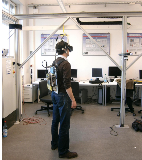
Fig. 1. User wearing the integrated tracking and visualization system. Vision is provided by an HMD, position and viewing direction are resolved according to the user's actual pose.
