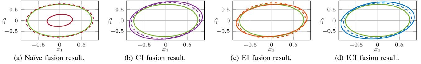
Fig. 5: Fusion results in node S5 at the end of the communication path in Fig. 4. The dashed ellipsoid represents the actual error covariance matrix, which is compared with the reported covariance matrix shown as solid ellipsoid. The green ellipsoid corresponds to the covariance matrix of the best attainable estimate provided by a centralized Kalman filter.
