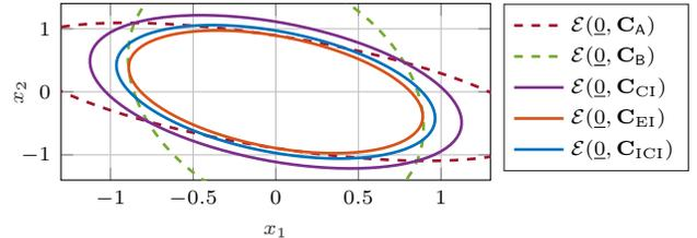
Fig. 1: Results of different fusion methods depicted as ellipsoids centered at origin. The ellipsoid related to CI is a bound on the intersection  $\mathcal{E}(\underline{0}, \mathbf{C}_A) \cap \mathcal{E}(\underline{0}, \mathbf{C}_B)$ . The ellipsoid related to EI is the largest ellipsoid inside the intersection. The ellipsoid for ICI lies in between those related to CI and EI.
