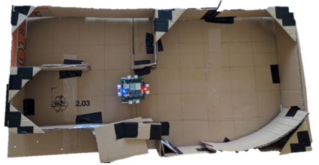
Figure 4: Robot navigating in the experimental setup. Using our proposed SLAM approach, the robot aims to estimate itself for both orientation and position in an unknown environment with surrounding cardboard obstacles.
