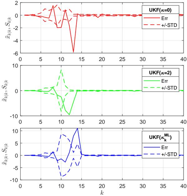
Figure 1. UKF performance depending on the scaling parameter setting.
