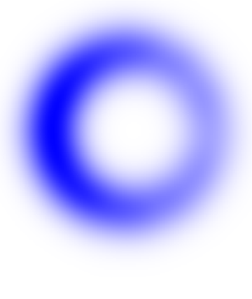
Fig. 3. Posterior density after one measurement update step. The measurement update produces a ring-shaped posterior density with higher likelihood around the target location.
