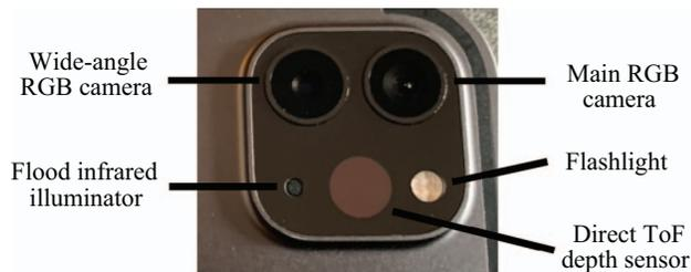
Fig. 3. Sensors on the back of the iPad Pro 2021. Width and height of the panel are around 27 mm.
