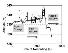
Fig. 4. Illustration of the fusion algorithm using the barometric sensor and building information
