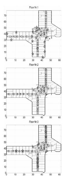
Fig.2. The test environment. The BSs are marked with pentagrams; the calibration points are marked with '+' and the test points are marked with 'o'.
