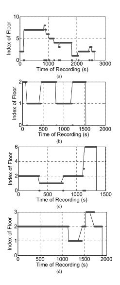
Fig.6. Floor estimation by adaptive calibration based algorithm. (a) - (d) correspond to the four measurement data sets in Figure 5 respectively. The lines stand for the real trace in floor level. The series of points stand for the estimated trace in floor level.
