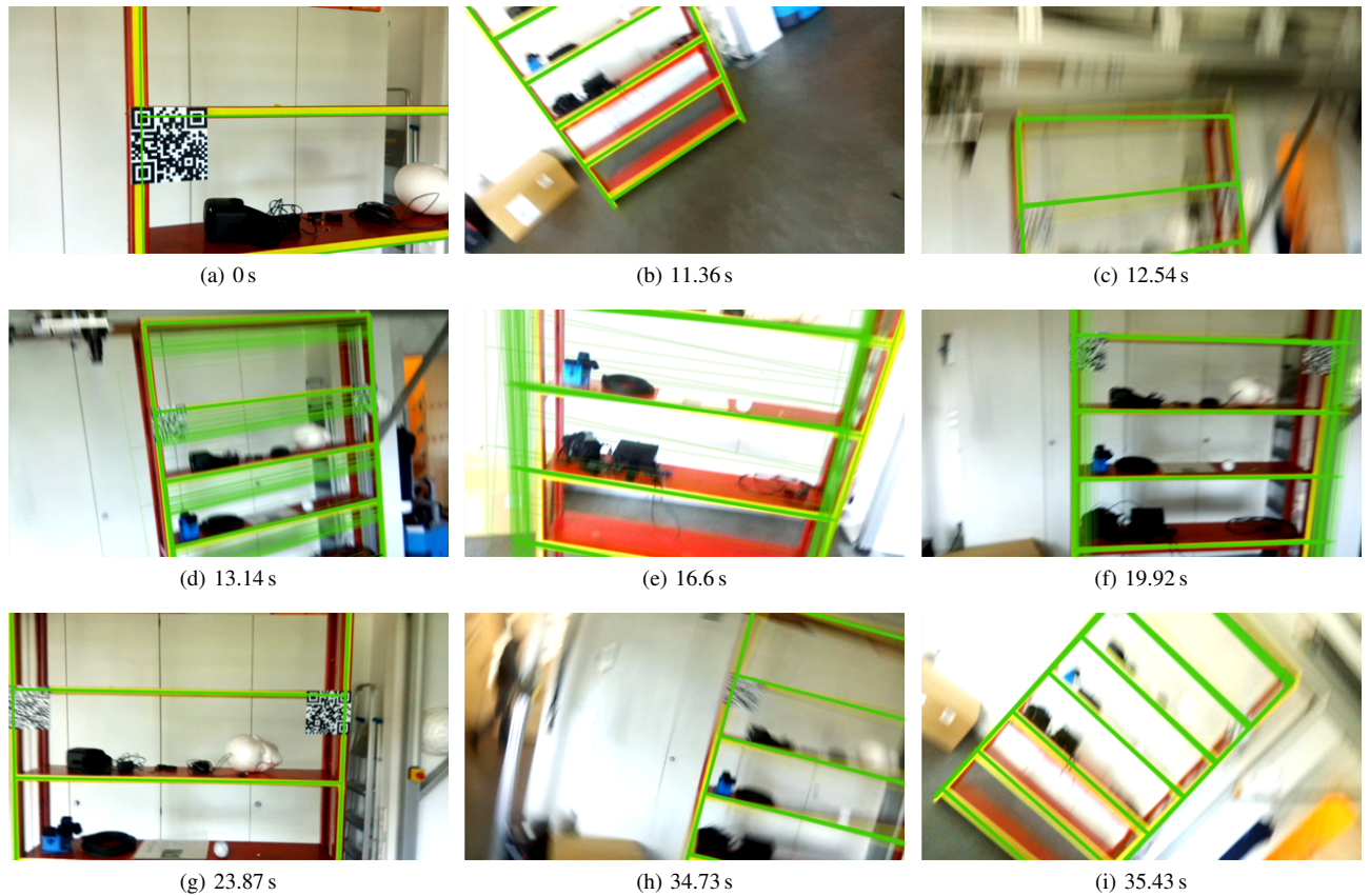
Fig. 6: Frames of test sequence, (a) initialization, (b,c) track kept with low variance under fast motion, (d-f) higher variance shortly after turn-away periods, (g-i) track kept with low variance under fast motion.
