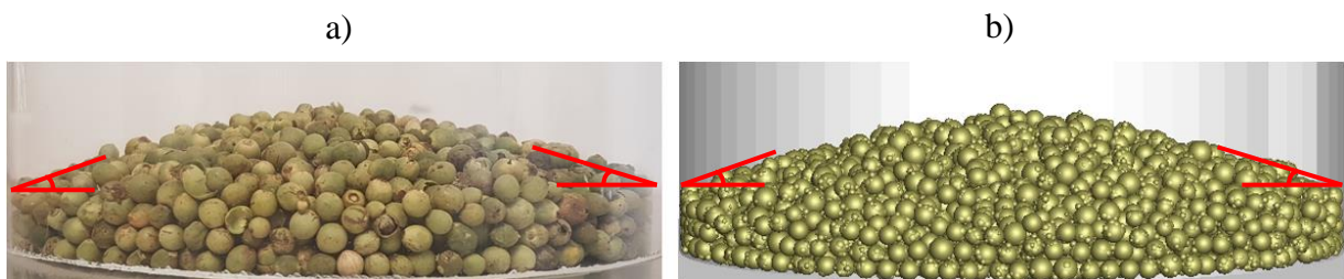
Figure 4: Angle of repose compared between a) experiment and b) simulation, static scenario
