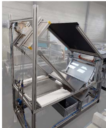
Fig. 2. Image of the sorting system. The material is fed into the system via a vibration feeder and a chute (on the right in the image). It is perceived by an area-scan camera, which is located at the top left of the image. Below the chute is an array of compressed air nozzles that separate the material.
