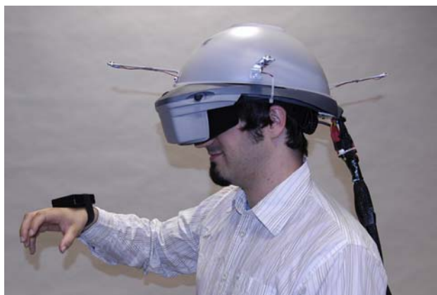
Figure 6: An operator with head-mounted display, head tracker and hand tracker.
