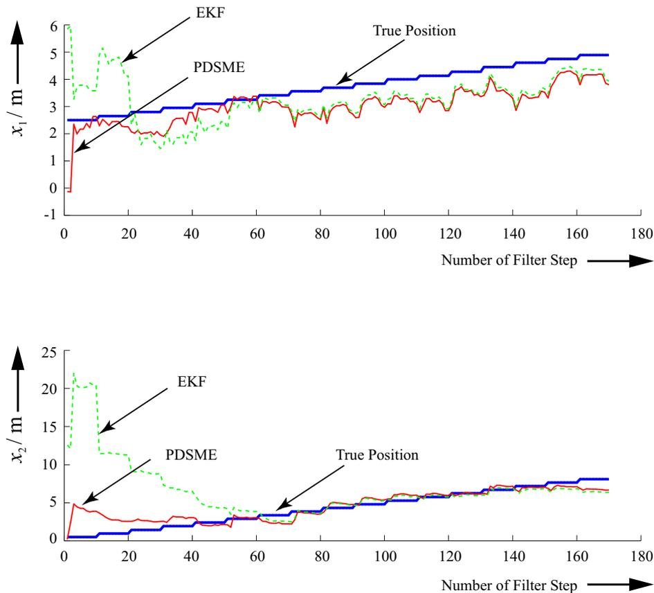
**Figure 7.** Comparison of the expected values of the estimated position calculated by the EKF (dashed lines) and the PDSME (thin solid lines) to the exact position (thick solid lines) for the  $x_1$  and  $x_2$  coordinates.
