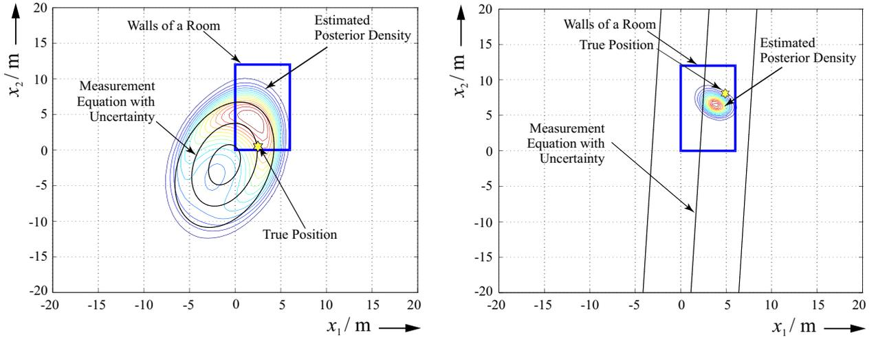
**Figure 6.** Localization with the PDSME: First filter step (left) and 170th filter step (right).
