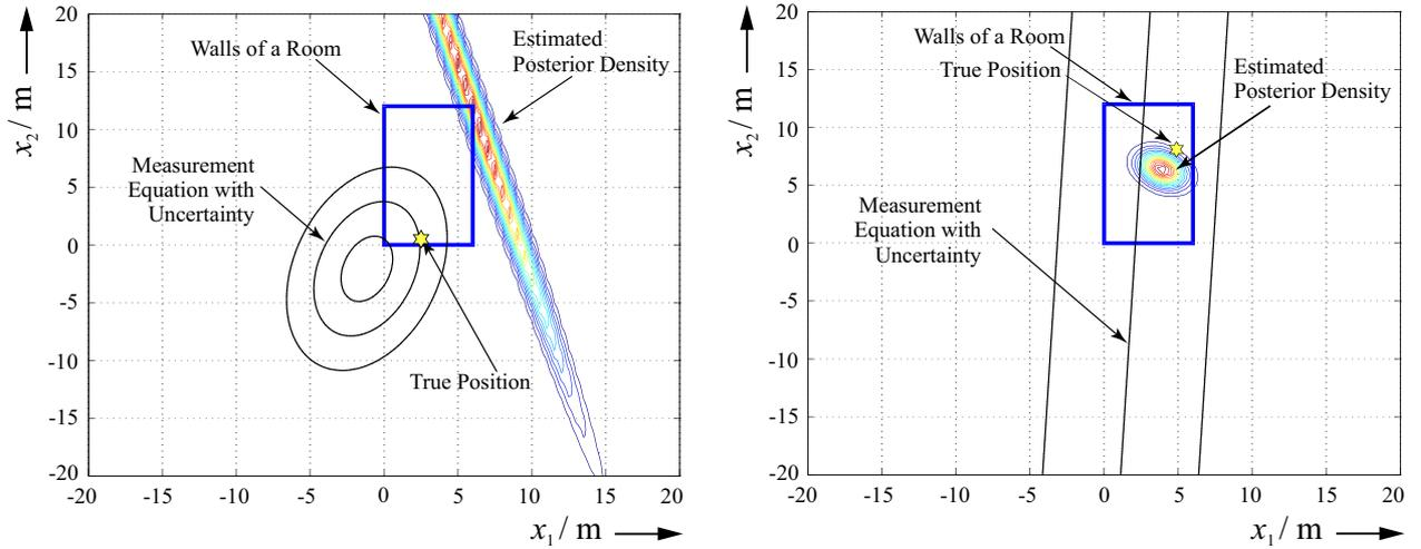
Figure 5. Localization with the EKF: First filter step (left) and 170th filter step (right).
