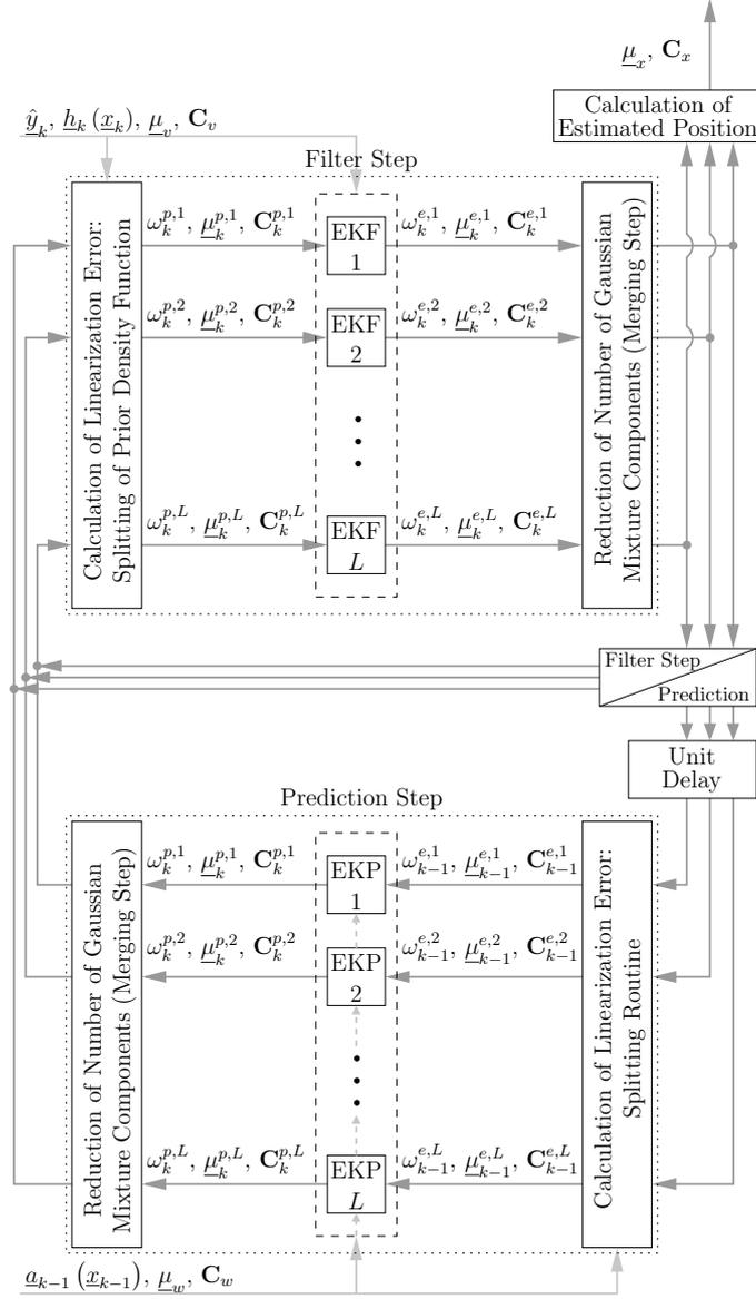
**Figure 3.** Overview of the PDSME algorithm: The PDSME consists of a linearized filter step (upper part) and linearized prediction step (lower part).
