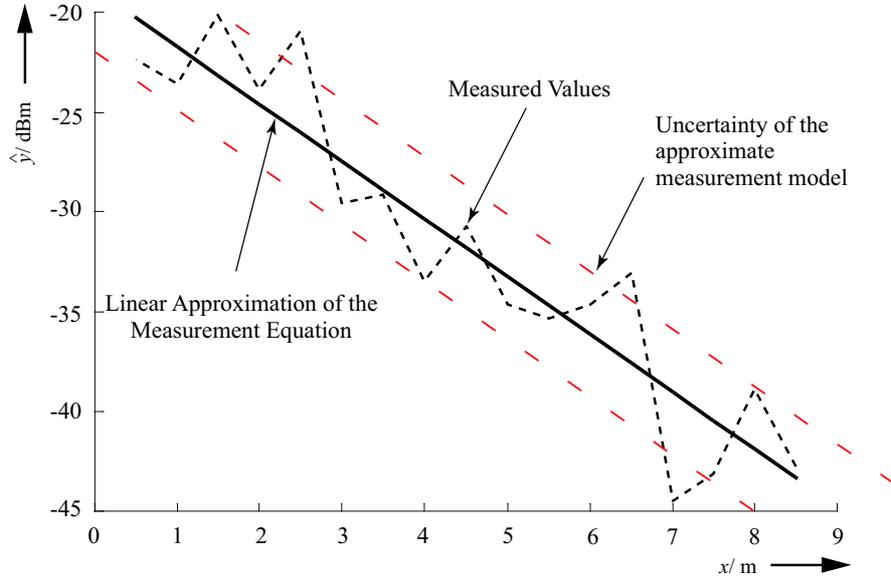
**Figure 1.** Assumed linear approximation of the measured logarithmic received signal power and uncertainties of the approximate measurement model caused by deviations between the measurements and the assumed measurement model.
