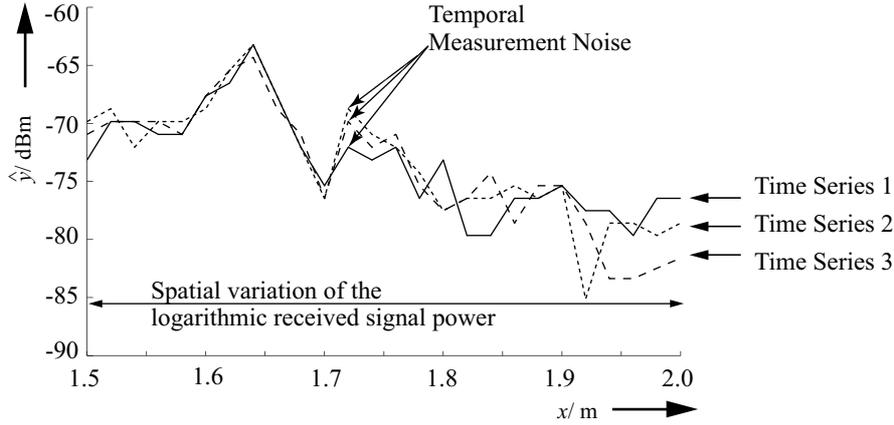
**Figure 2.** Spatial variations of the logarithmic received signal power over short distances and temporal measurement noise (three different time series).
